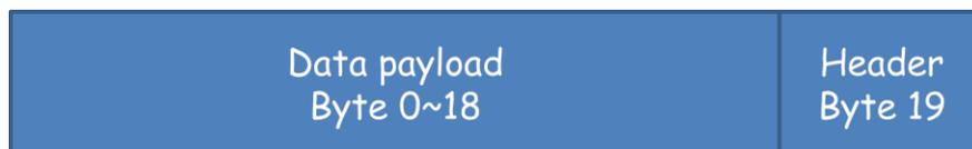
The Header is composed of two elements. The one is length of data payload. The other is packet index. If the payload isn't the last one, the packet index is "0". If the payload is the last one, the packet index is "0x80".
