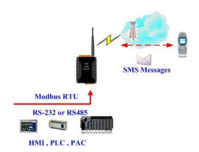
(2) The host needs to send the SMS content command to define the variable part of the alarm SMS first. Then, send the transmitting SMS command.
