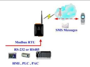
(2) The host can send the Modbus command periodically to inquire the GT-531 whether has received the SMS. If the GT-531 has received the SMS, you can send the command to read it.
