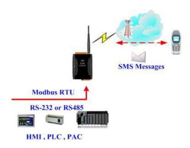
(2) Sending the Modbus commands from the Host to the GT-531 to transmit the alarm SMS as follows:
