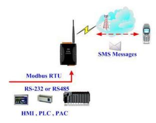
(2) The host sends the Modbus commands to the GT-531 to set the content of the SMS and phone number first. Then, send the command to transmit the SMS.
