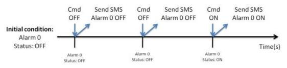
2. Edge Trigger mode : Triggered when the state changes.
