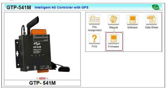
4. After downloading the firmware to be updated, put the file into the "update" folder of the SD card and rename the firmware file to "fw".
