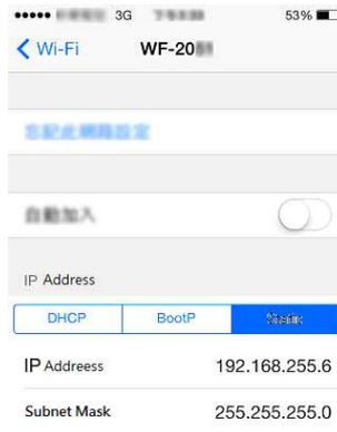
d. After the above settings, you can use your Smartphone to connect to the WF-2000 (IP address "192.168.255.1")
